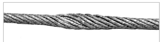
The wire rope is flattened at one point. This can result, for example, from the wire rope being pinched.
