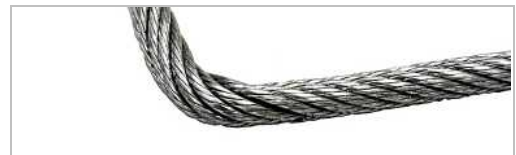
There is a kink in the wire rope. This can result, for example, from violent external forces being applied to the wire rope.
