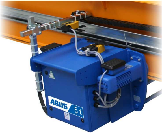
Cross-type limit switch as trolley travel limit switch
